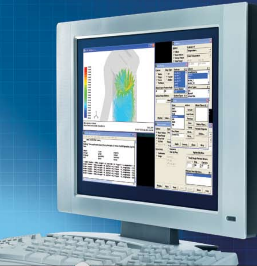
Temperature profiles indicating gas cooling using FloMax® air atomizing nozzles inside the tower.
